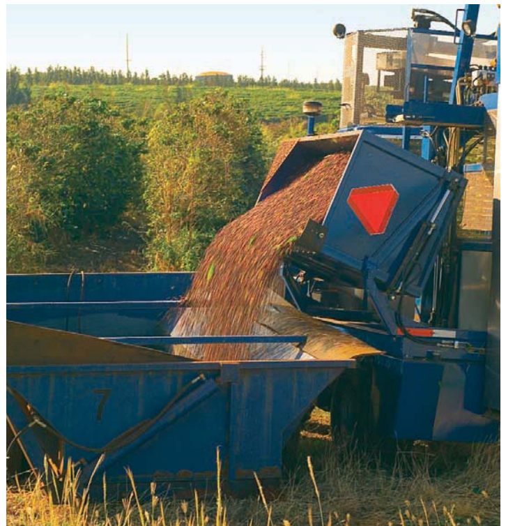
Coffee plants are harvested for their cherries once a year, starting around September. A machine designed for coffee harvesting shakes the branches to release the fruit.
